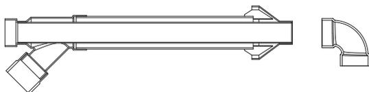
From inside the building, insert the outer, straight combustion air-inlet pipe through the weather-seal boot flashing so that the height from the roof to the rear of the rain cap when installed is as specified in the subsequent diagrams.
