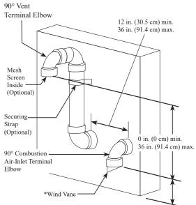
\*For installations using 3 in. (7.6 cm) pipe and fittings, a 90 elbow equipped with a wind vane deflector must be used for the combustion air-inlet terminal. Contact Manufacture's National Service Department for the elbow.
