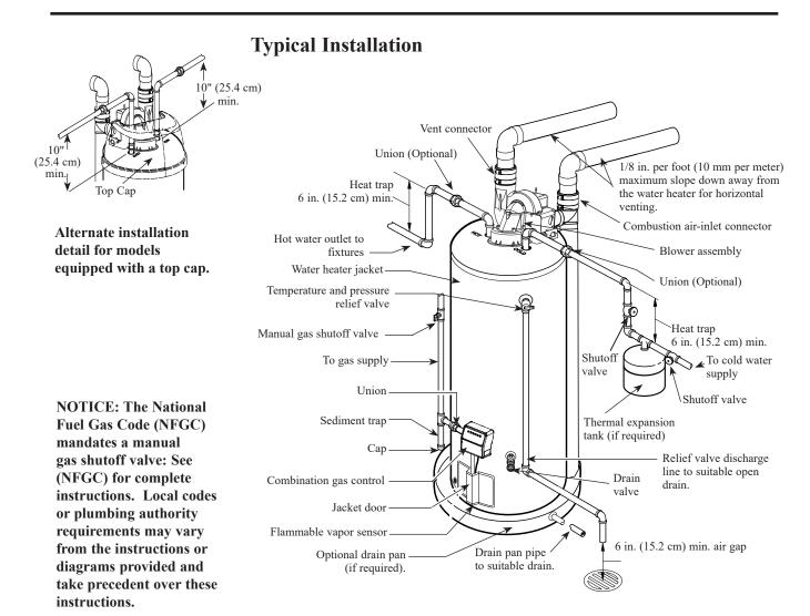
A new combination temperature and pressure relief valve, complying with the current Standard for Relief Valves for Hot Water Supply Systems, ANSI Z21.22 /CSA 4.4, is factory installed and must remain in the opening provided and marked for the purpose on the water heater. No valve of any type should be installed between the relief valve and the tank. Local codes shall govern the installation of relief valves.
