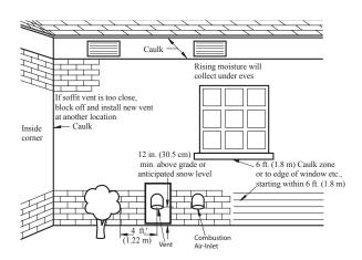
AWARNING: Moisture in the flue gas will condense as it leaves the vent terminal. In cold weather this condensate can freeze on the exterior wall, under the eaves and on surrounding objects. Some discoloration to the exterior of the building is to be expected. However, improper location or installation can result in severe damage to the structure or exterior finish of the building
