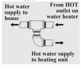
Tee fitting for horizontal hot water supply lines.
