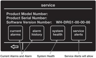
History allows you to access any current alarms that have been tripped and view a list of previous alarms. system Health will show you the status of the tank's combustion health and overall tank health. Service Alerts will allow you to set how often you want to be alerted to check venting, clean the drain trap, replace the neutralizer, and to drain and inspect the tank.
