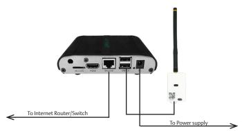
• Plug the Server into an electrical outlet with the supplied power cord.
