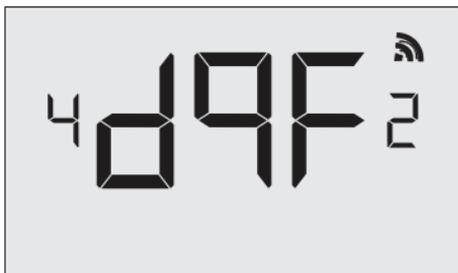
Each wireless thermostat must be paired with an individual HVAC Controller during installation. The thermostat will search for the closest HVAC Controller to it and display the unique HVAC Controller ID. The HVAC Controller ID is located on the case of the HVAC Controller. **Only install one room at a time.**
