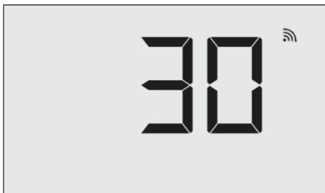
The thermostat will countdown from thirty (30) seconds. If the sensor has successfully paired, the thermostat will display *SUCC*. If the sensor did not pair successfully, the display will read *FAIL*, and the process must be repeated.
