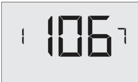
**62-82** (67°F\* default setting) Select the room temperature in °F that a HVAC unit will have to attain within the selected “Temperature Recovery Time” when there is a need for heating.
