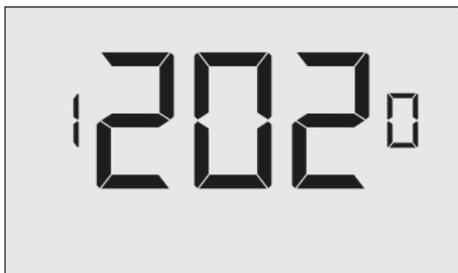
**00-120** (20\* default setting) Select the time delay (in minutes) for which the room that is in the guest occupancy mode needs to be unoccupied before the temperature setback is initiated.
