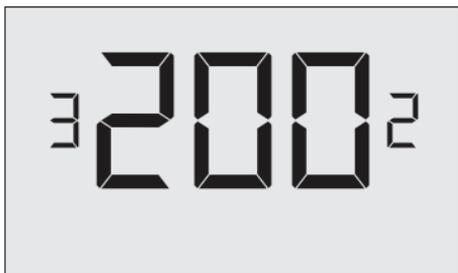
**02-08** (2°F\* default setting) Select the °F differential between Low Fan and 2nd stage fan (Medium or High) when Auto-Fan Speed is selected.
