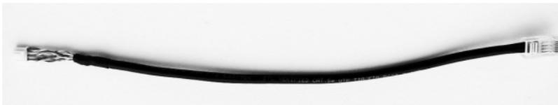
Connect the J4 harness into the J4 port on the right side of the wireless controller.
