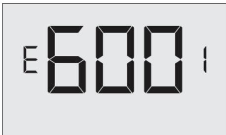
**00-60** (01\* default setting) Select the minimum period of time (in minutes) for which occupancy needs to be detected in order to consider the room occupied during the “Night Occupancy” period.
