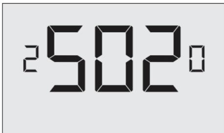
**05-30** (2.0°F\* default setting) Select the °F differential required to trigger 2nd stage cooling ().
