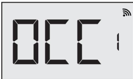
The thermostat allows the user to choose the functionality of a sensor. Use the table below to configure the desired functionalities. For example, if sensor is intended to be used as Occupancy Sensor, OCC value must be set to 1.
