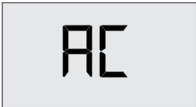
After you have entered the equipment code, the t-stat will ask you for the source of the temperature reading. Temperature can be sensed by the thermostat (TS) or by a conditioning unit (AC) if a conditioning unit supports the option of reading temperature.
