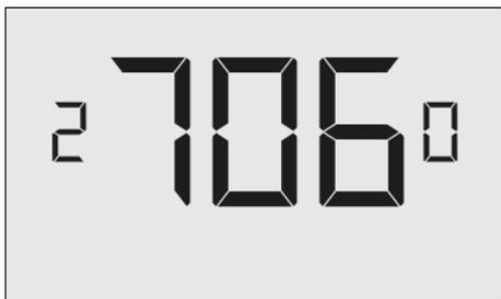
**55-70** (60\* default setting) Select the relative humidity level that automatic humidity control will attempt to control for in conjunction with the humidity cut-off temp.
