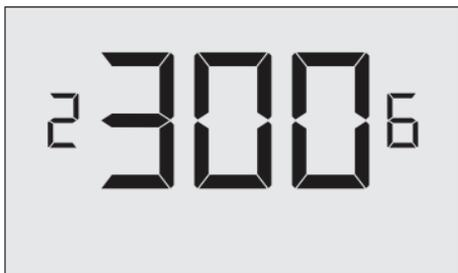
**04-20** (0.6°F\* default setting) Select the °F of overshoot above or below the setpoint on the thermostat before the thermostat stops the call for cooling or heating.
