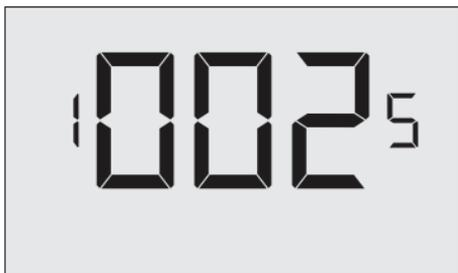
**00-60** (25\* default setting) Select the maximum time allowed for a HVAC unit to attain temperature as defined by Heat and Cool “Recovery Temperature”;
