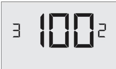
**01-60** (2\* default setting) Select the time delay (in minutes) before the thermostat disables air conditioning when a door or window sensor has been installed.
